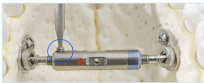
The blocking screw (D002) is placed in one of the two available threaded holes with the screwdriver (IT0128). Place the blocking screw perpendicular over the cylinder, with a clear view of the screw hole. The blocking screw should be fixed real firm, using wrist force.
